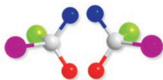
Fig. 6.7: A chiral molecule and its mirror image
